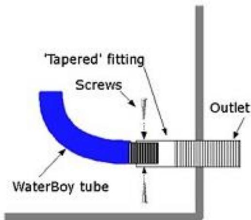
If the connection is still incompatible then most likely the tank has a 'tapered' thread which is illustrated in the diagram to the left. If this is the case, you should use the 2 screws included with the WaterBoy packing it if necessary with insulation tape or similar and then screwing through the taper into the Waterboy end fitting. The main requirement is a reasonably firm fit by whatever means possible.
